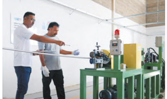
Stahlmann corrugated tube fed for annealing
